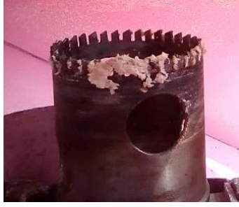
a. Remaining starch stuck on the saw-tooth blade after cutting
