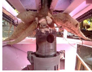
b. Incomplete-cut tubers
