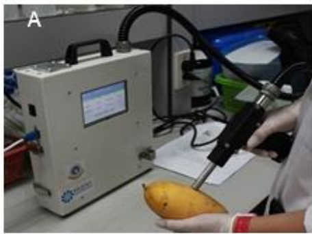
Figure 1 Mango fruit spectra acquisition using two NIR spectrometers: portable (A) and commercial (B)
