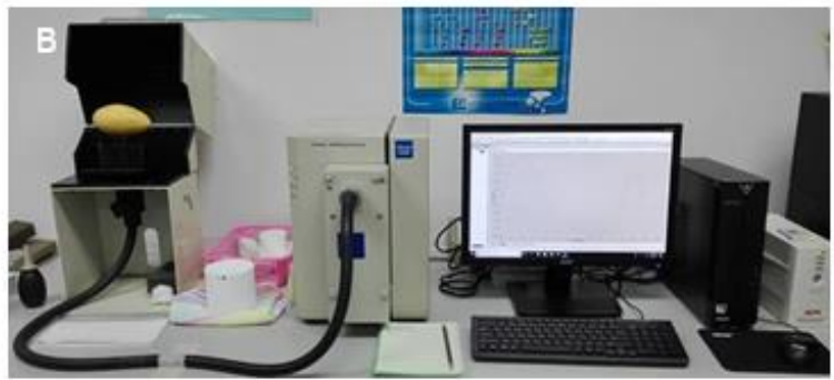
Figure 1 Mango fruit spectra acquisition using two NIR spectrometers: portable (A) and commercial (B)
