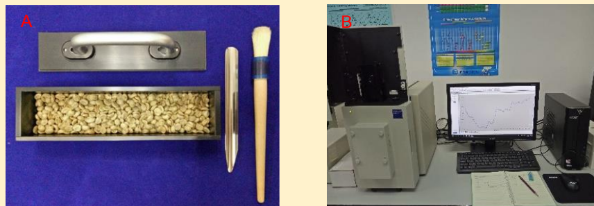
Figure 1 Green coffee bean packing in coarse sample cell (A) for NIR spectra measurement by NIRSystem 6500 (B)
