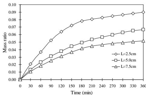
Figure 5 Adsorption performance of desiccant unit with different tray thickness.
