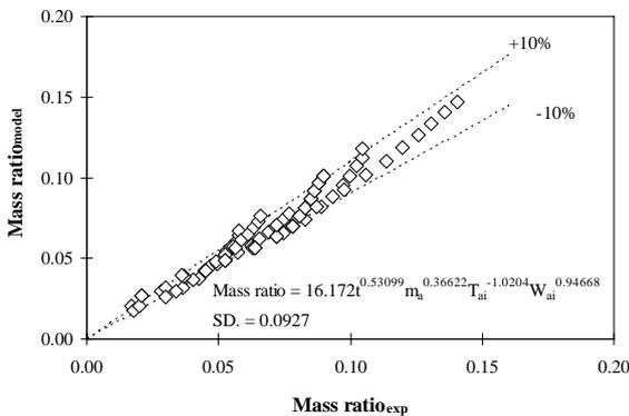
Figure 15 Comparisons of mass ratio calculated from the experimental data and model in case of adsorption process.
