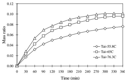
Figure 13 Regeneration performance of desiccant unit with difference air inlet temperature.
