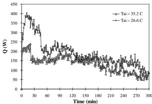
Figure 11 Heat transfer rate from adsorption process with different air inlet temperature.
