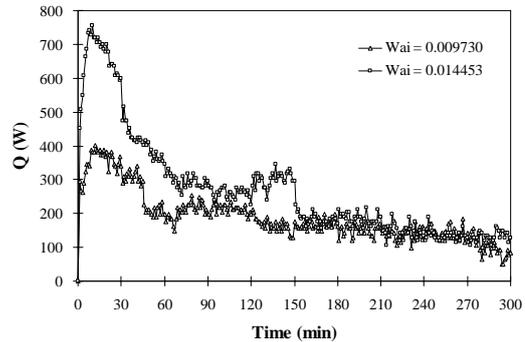
Figure 12 Heat transfer rate from adsorption process with different air moisture content.
