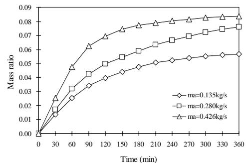
Figure 14 Regeneration performance of desiccant unit with difference mass flow rate of air.
