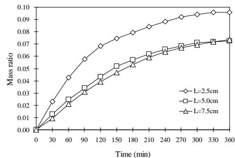
Figure 6 Regeneration performance of desiccant unit with different tray thickness.
