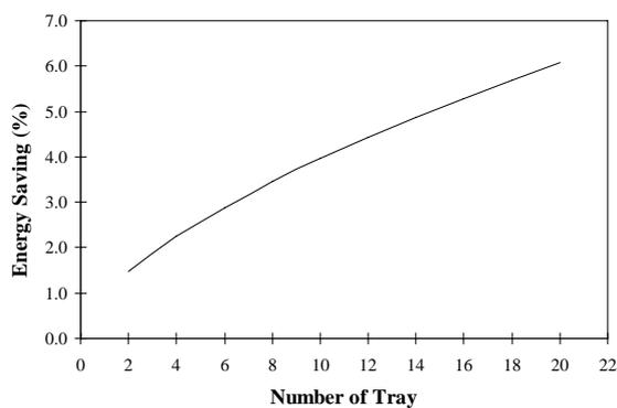
Figure 20 Energy saving at various numbers of trays.
