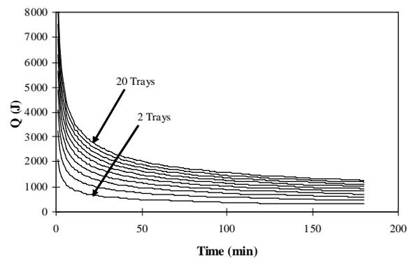
Figure 19 Heat transfer rate from adsorption process by silica gel at various times.
