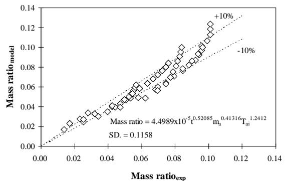
Figure 16 Comparisons of mass ratio calculated from the experimental data and model in case of regeneration process.
