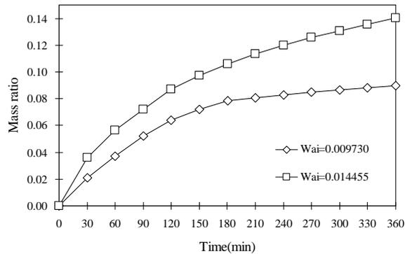
Figure 9 Adsorption performance of desiccant unit with difference moisture content in air.
