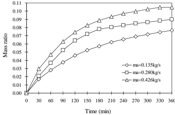
Figure 7 Adsorption performance of desiccant unit with difference air mass flow rate.
