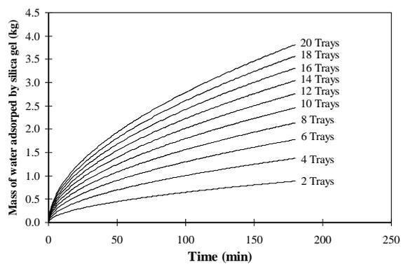
Figure 18 Mass of water adsorbed by silica gel at various times.
