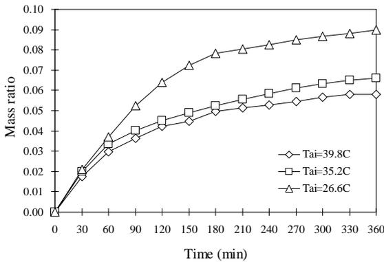
Figure 8 Adsorption performance of desiccant unit with difference air inlet temperature.
