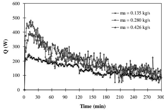
Figure 10 Heat transfer rate from adsorption process with different mass flow rate of air.
