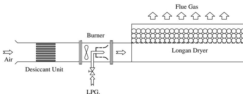
Figure 3 Longan dryer with desiccant unit.
