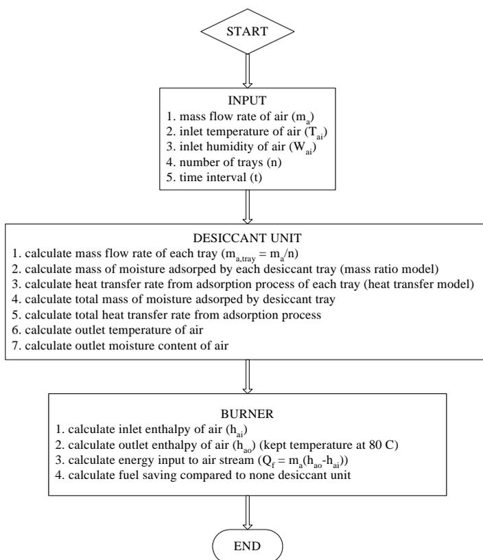
Figure 4 Flow chart for evaluating the energy saving of longan dryer having desiccant unit.
