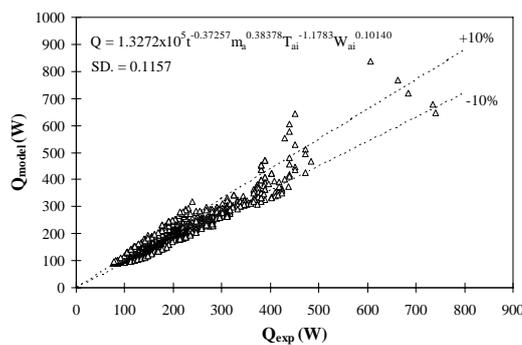
Figure 17 Comparisons of heat transfer rate calculated from the experimental data and model.
