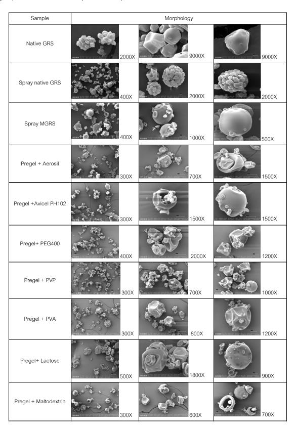
Figure 1 The morphology of modified glutinous rice starch with various additives
