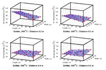
Figure 2 Surface plot of air temperature distributions (°C) and emitter temperature (constant at 800 °C) at different distances between emitter and absorbing surface (0.20, 0.30, 0.40 and 0.50 m) versus absorbing area of radiant distribution (width (m), length (m)).
