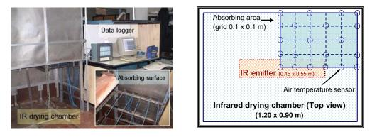
Figure 1 (a) Gas-fired infrared dryer; (b) Installation of air temperature sensor on tray which was designed as grid.
