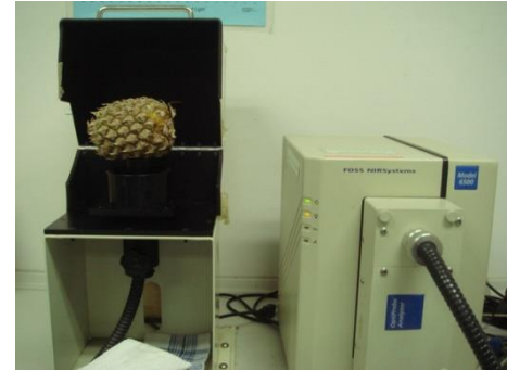
Measuring NIR spectrum by NIRSystem 6500
